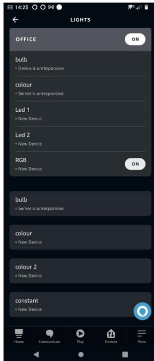
You can control the receivers through an Amazon Alexa using voice commands to set the lighting level as a percent, set the lights to on or off, and to set the colour of RGB enabled receivers.
