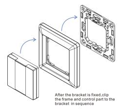
The key part of this controller is a universal, standard size design switch element that can be integrated in numerous frames by different manufactures as below list:
