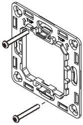
**Method 2:** Screw the bracket to the wall
