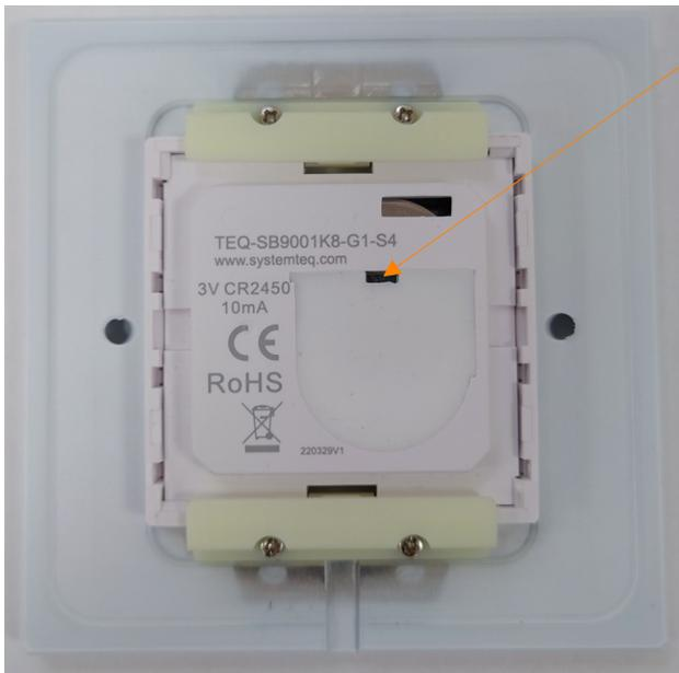
Open the battery compartment and remove the plastic blocker to enable the battery to power the switch plate, then cover the compartment back up.
