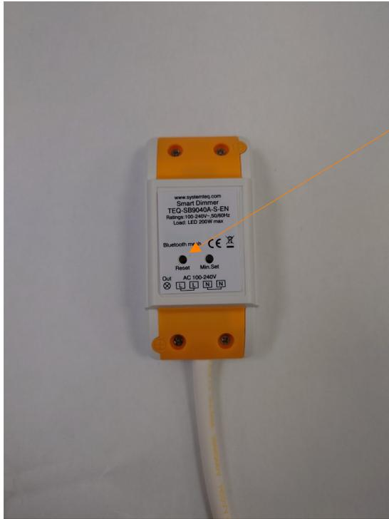
While the device is scanning, press the program button on the receiver twice. In the case of our smart dimmer, this is the reset button.
