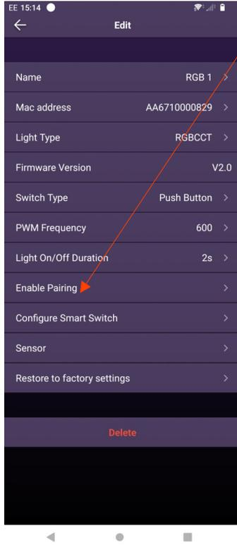
You will have a 4 second countdown on screen, during which time you must press the “on” button on the switch plate to pair the receiver.
