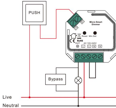
**NOTE:** Switch connected to the S1 terminal activates the basic functionality of the dimmer (turning the light on/off, dimming).
