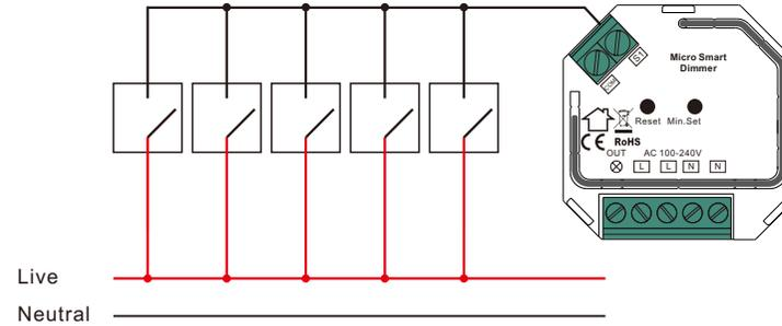
This phase dimmer adopts leading edge dimming (forward phase control) or trailing edge dimming (reverse phase control), two versions are available for choosing, factory default version is trailing edge. Please make sure the connected loads support the control type you choose. Please refer to the user manual of the load or consult the supplier of the load.
