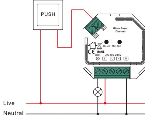
**NOTE:** Switch connected to the S1 terminal activates the basic functionality of the dimmer (turning the light on/off, dimming).
